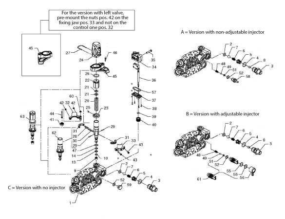
\* When assembling apply petroleum based grease
