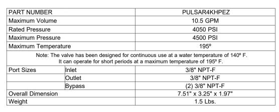
General Pump recommends using a safety relief device in conjunction with this unloader valve when installed on a positive displacement pump. General Pump is not liable and assumes no responsibility when used in a customer's high pressure system.
